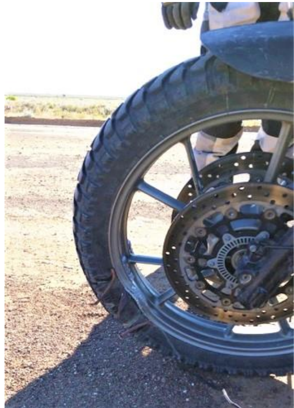
Figure 4 - a successful 'plug' to a damaged tubeless rim after the rider hit a rock in a dry creek crossing on the Birdsville Track
