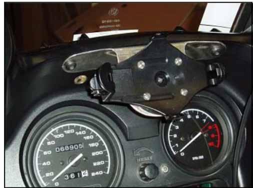
Stainless steel mount shaped to fit the bike with part of the standard 276C marine mount screwed to it.
