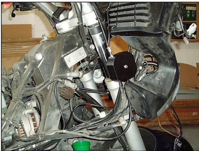
Vacuum actuator mounted just behind the oil cooler.
